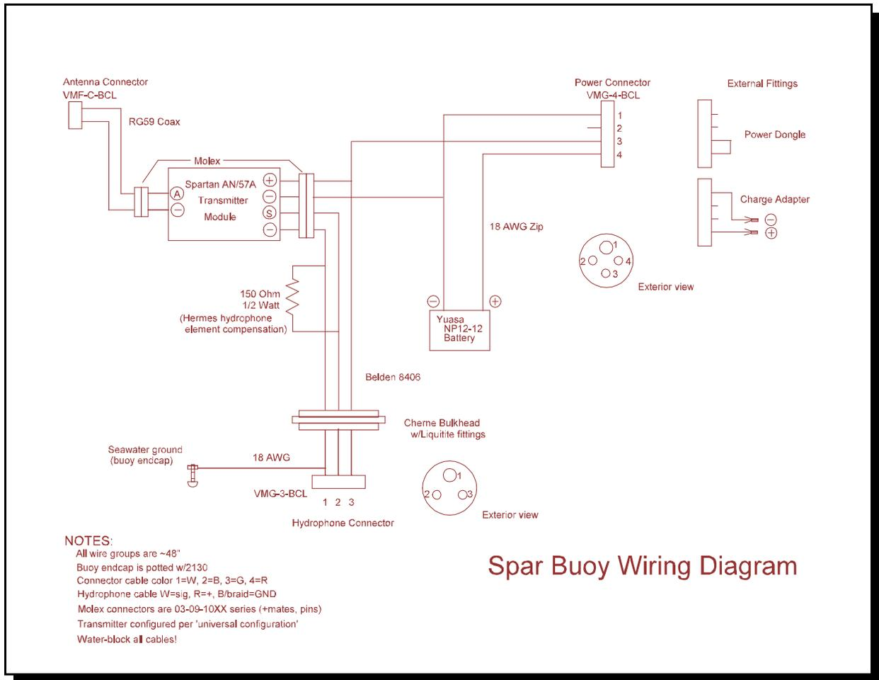
**Figure 5. Wiring**
